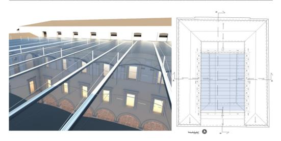
Figure 3: Rendered image of the ETFE roof seen from the top (left), installation of the ETFE roof (right).
