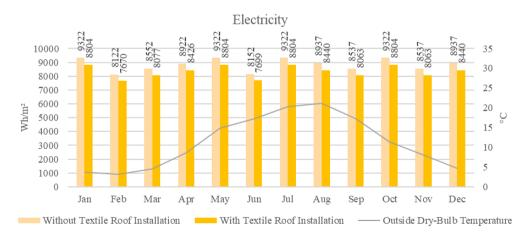
Figure 5: Chart showing the Electricity consumption levels in the building during 12 months without the textile roof installation and with it.
