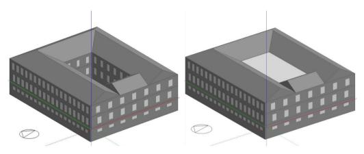
Figure 4: Design Builder model of the building without the ETFE courtyard covering (left) and with the ETFE courtyard covering (right).
