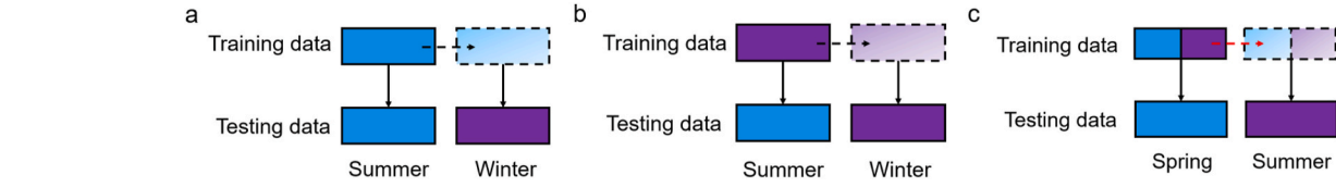
Fig. 11. The proposed data experiments under the NREL's fault dataset: (a) Training data: the summer dataset; testing data: each season's dataset. (b) Training data: the winter dataset; testing data: each season's dataset. (c) Training data: a mixed dataset of summer and winter of half size from each; testing data: each season's dataset.
