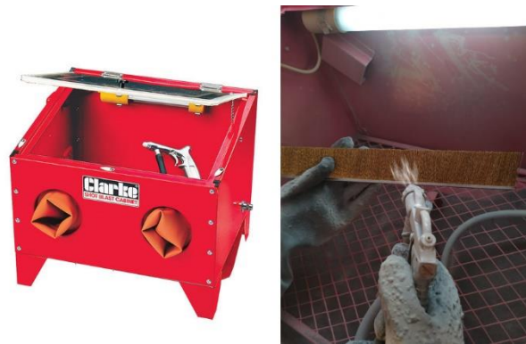
Figure 9: Heavy duty sand blasting chamber (left). Sand blasting of a brush (right).
