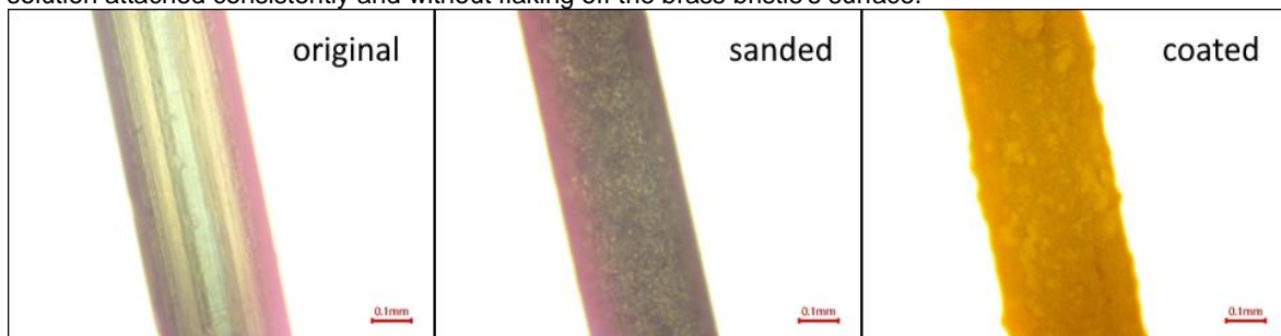
Figure 11: Microscopic surface comparison of a brass bristle.
