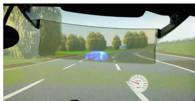
Figure 8. Internal view of the HUD and virtual car imagery demonstrated
