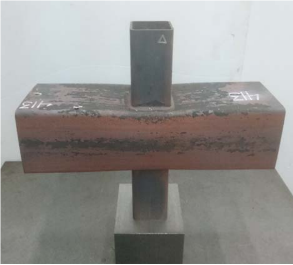
(c) Test vs FE comparison for RHS X-joint (X8) with \psi = 750^\circ\text{C} and failed by F mode.
