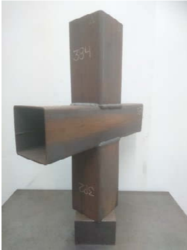
(a) Test vs FE comparison for RHS X-joint (X3) with \psi = 300^\circ\text{C} and failed by S mode.
