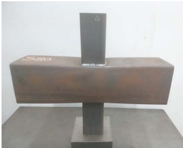
(a) Test vs FE comparison for RHS X-joint (X2) with \psi = 300^\circ\text{C} and failed by F mode.
