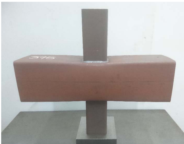
(b) Test vs FE comparison for RHS X-joint (X5) with \psi = 550^\circ\text{C} and failed by F mode.
