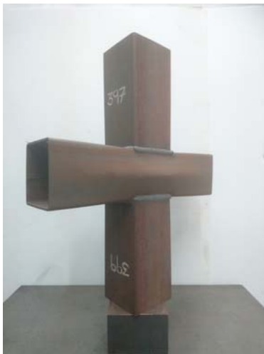
(b) Test vs FE comparison for RHS X-joint (X6) with \psi = 550^\circ\text{C} and failed by S mode.
