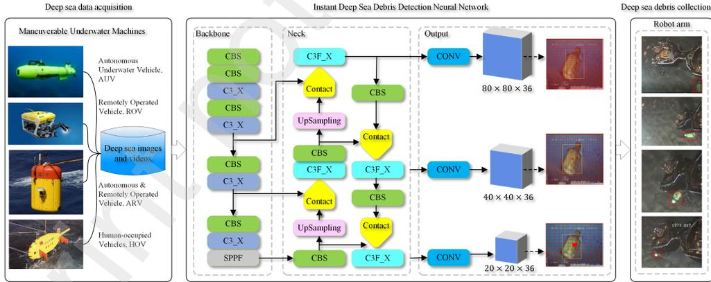
Figure 3: The workflow of the proposed methodology to detect and clean deep sea debris with DSDebrisNet for maneuverable underwater machines.
