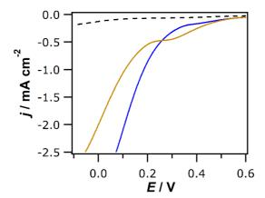
**Figure S6.** Voltammograms of O<sub>2</sub>-saturated [dema][TfO] before and after heating to 150 °C for 64 hours recorded using a Pt-disk electrode rotating at 1,600 rpm. The dashed black line shows the voltammogram of Ar-saturated [dema][TfO] before heating. Each voltammogram was recorded at 100 mV s<sup>-1</sup> and the sweep was in the negative direction.
