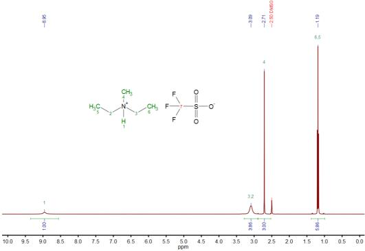
Figure S8. <sup>1</sup>H NMR spectrum of [dema][TfO] containing 11.7 ppm H<sub>2</sub>O.
