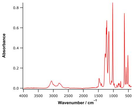
**Figure S7.** FTIR-ATR absorbance spectrum of [dema][TfO] containing  $\approx$ 11.7 ppm H<sub>2</sub>O recorded at 30 °C
