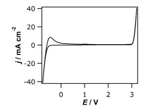
**Figure S2.** Cyclic voltammogram of [dema][TfO] ( $\approx 8$  ppm H<sub>2</sub>O) recorded using a Pt working electrode. The potential cycles begin in a negative-going direction at 100 mV s<sup>-1</sup>. Below -0.8 V the [dema]<sup>+</sup> cation is reduced to H<sub>2</sub> and dema. Electrogenerated H<sub>2</sub> is oxidized in the forward sweep at about -0.5 V. At positive potentials, the [TfO]<sup>-</sup> anion is oxidised.
