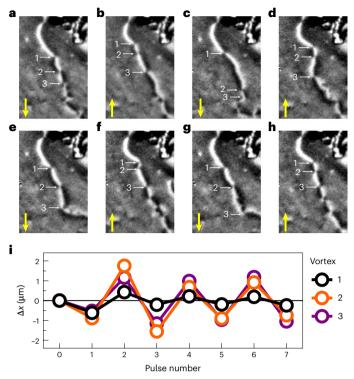
Fig. 3 | Movement of meron-antimeron pairs using electrical pulses. a-h, XMLD-PEEM images of the  $180^\circ$  AFDW after applying successive 1 ms, 21 V electrical pulses in the directions indicated by the yellow arrows. The width of each image corresponds to  $1.2 \, \mu m$ . i, The average displacement of vortices 1 to 3 indicated in a, measured after each pulse.
