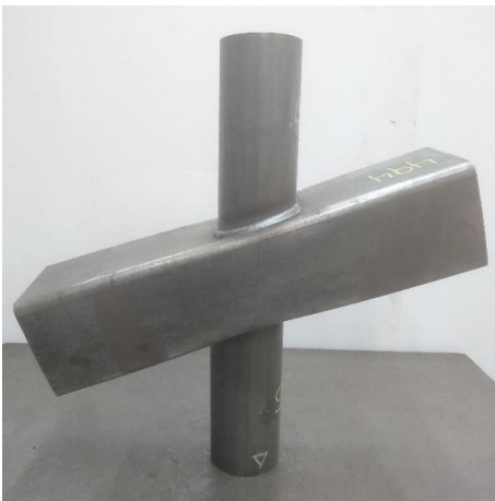
(b) Comparison of test and FE 50° CHS-to-RHS X-joint failed by F mode.
