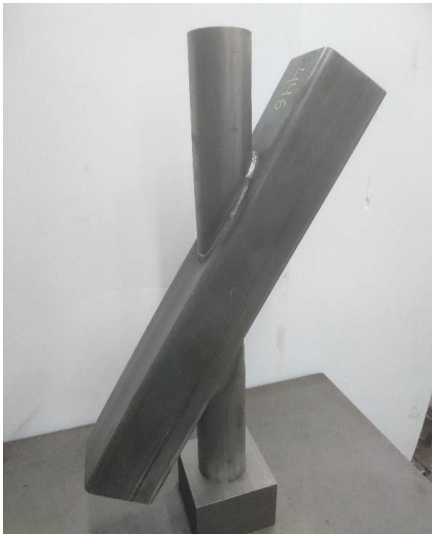
(a) Comparison of test and FE 30° CHS-to-RHS X-joint failed by F mode.
