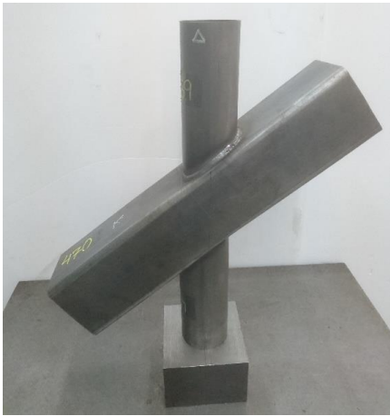
(b) Comparison of test and FE 50° CHS-to-RHS X-joint failed by F mode.
