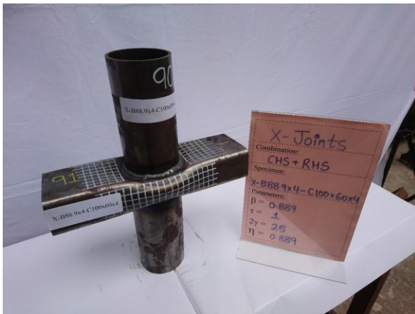
(b) Comparison of test and FE 90° CHS-to-RHS X-joint failed by F+S mode.
