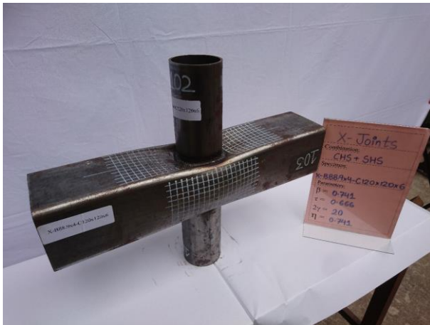
(a) Comparison of test and FE 90° CHS-to-RHS X-joint failed by F mode.
