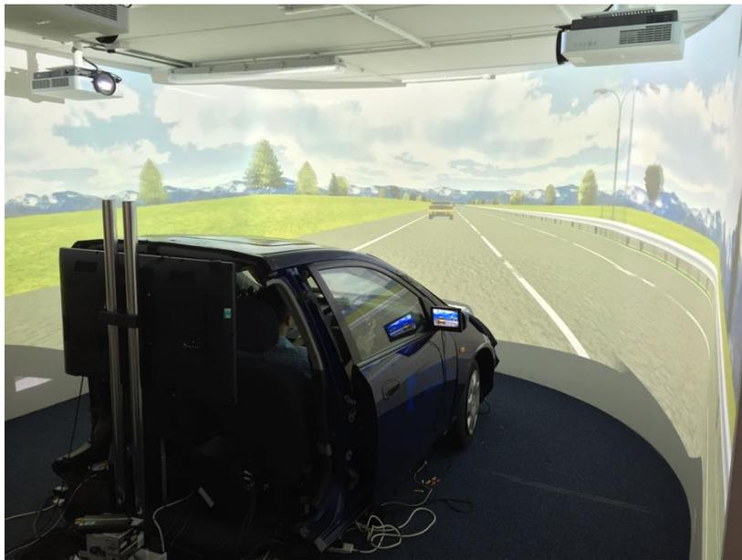
**Figure 1 - Medium fidelity driving simulator showing motorway scenario used during study**
