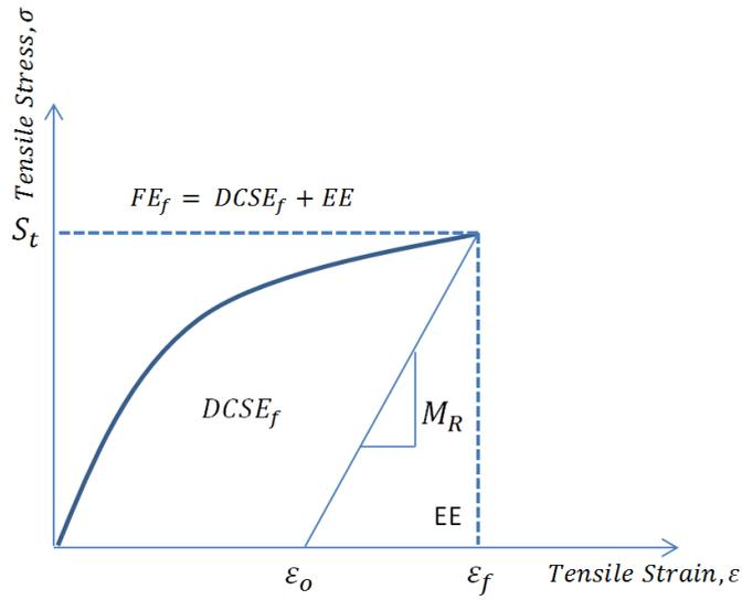
Fig. 7. Tensile strength versus tensile strain plot
