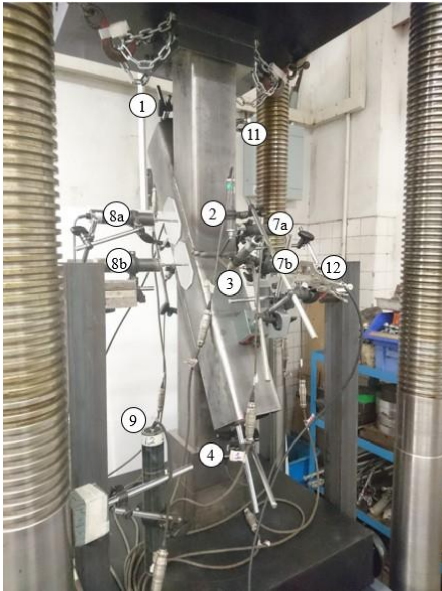
Fig. 16. Photo of tubular non-90° X-joint test setup in 5000 kN machine
