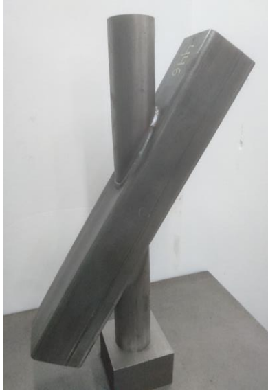
a. Chord face failure mode (F) of X-88.9×4-120×120×6-30°
