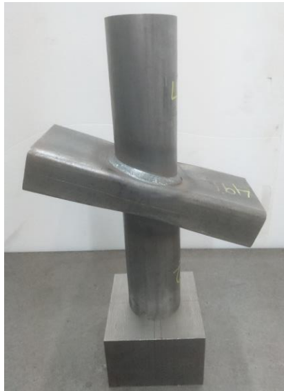
b. Chord face failure mode (F) of X-88.9×3-120×60×4-70°-R Fig. 25. Observed failure mode of CHS-RHS non-90° X-joints
