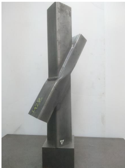
c. RHS-RHS non-90° X-joint failed by combined failure mode (F+S)
