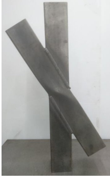
b. RHS-RHS non-90° X-joint failed by chord side wall failure mode (S)
