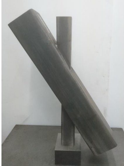
a. RHS-RHS non-90° X-joint failed by chord face failure mode (F)
