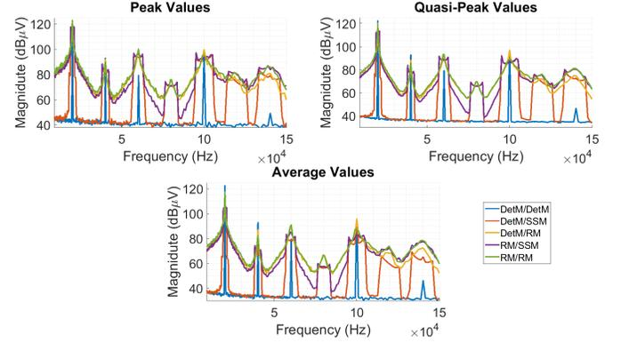
Fig. 8: Frequency-domain graphs obtained with the EMI receiver [9 kHz - 150 kHz]
