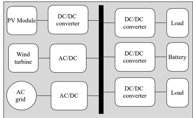
Fig. 1: Typical DC Microgrid set-up with the PCC [1]
