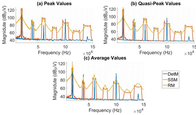
Fig. 6: Frequency-domain graphs obtained with the EMI receiver [9 kHz - 150 kHz]
