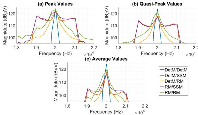
Fig. 7: Frequency-domain graphs obtained with the EMI receiver [18 kHz - 22 kHz]
