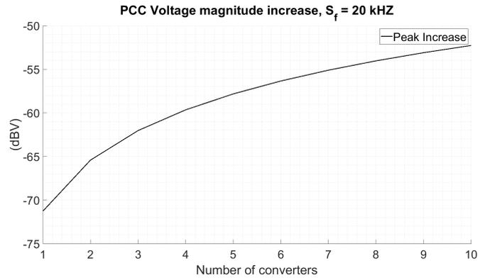
Fig. 2: Spectral aggregation of ten identical converters,  $S_f$  stands for switching frequency
