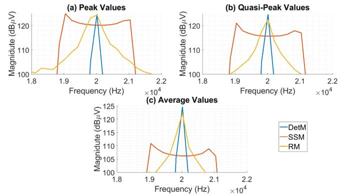
Fig. 5: Single converter: frequency-domain graphs obtained with the EMI receiver [18 kHz - 22 kHz]
