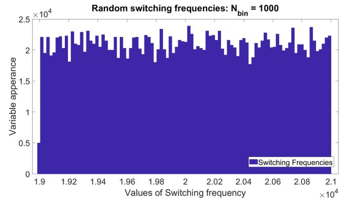
Fig. 3: Random switching frequencies generated by the PWM
