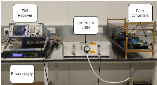
Fig. 4: Experimental test set-up
