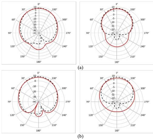
Fig.9. Comparison of the normalised radiation intensity in E- and H-plane of the antenna bent over 65° (red lines) with the radiation profiles of the flat antenna (black dashed lines), when the antenna is bent along (a) its length (E-plane bending), (b) its width (H-plane bending).
