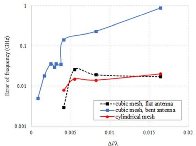
Fig.4. Illustration of the resonant frequency convergence with the mesh refinement when the cubic mesh is used for the flat antenna (light blue line), and for the bent antenna under the angle of  $18^\circ$  (blue line), and cylindrical mesh (red line) is used for the flat/bent antenna ( $\Delta l$  represents the observed cell size, and  $\lambda$  is the wavelength corresponding to the operating frequency).
