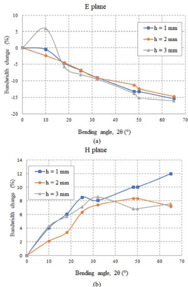
Fig.8. Bandwidth change for the case of a) E-plane bending and b) H-plane bending of antennas on the substrate thickness  $h=1, 2,$  and  $3$  mm.
