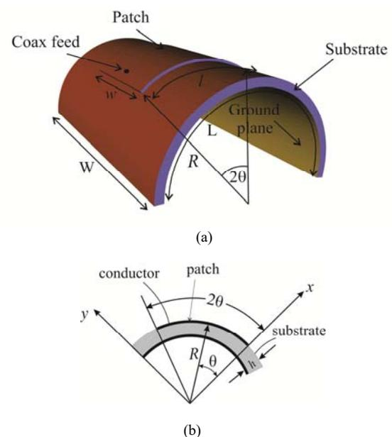
Fig.1. A cylindrically bent antenna (a) the geometry of the antenna bent in the E-plane; (b) the cross-section of the cylindrically bent antenna.
