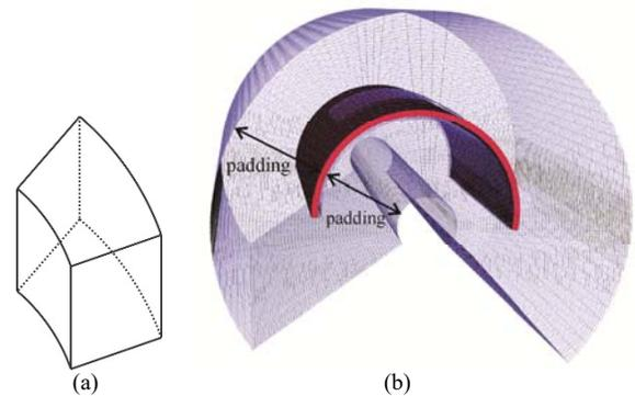
Fig.2. An antenna model in a cylindrical grid, (a) a cylindrical TLM cell, (b) the geometrical representation of the antenna bent in the E-plane inside the computational box.
