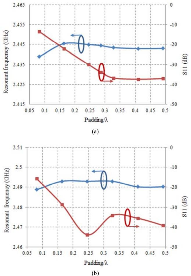
Fig.3. Comparison of the resonant frequency and  $S_{11}$  parameter of the flat antenna with  $h = 2$  mm substrate thickness for different padding values around the basic structure ranging from 10 mm to 60 mm (e.g.,  $0.08\lambda - 0.5\lambda$ ): (a) the cylindrical mesh, (b) the cubic mesh.
