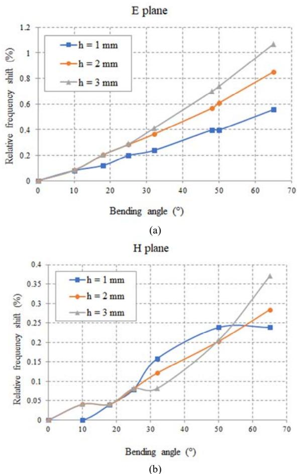
Fig.7. Relative resonant frequency shift for the case of a) E-plane bending and b) H-plane bending of antennas on the substrate of thickness  $h=1, 2,$  and  $3$  mm.
