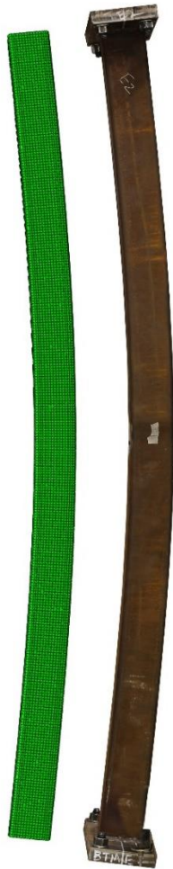
Fig. 6. Comparison of test and FE global buckling failure mode for H80×80×4-BC-e40 long beam-column
