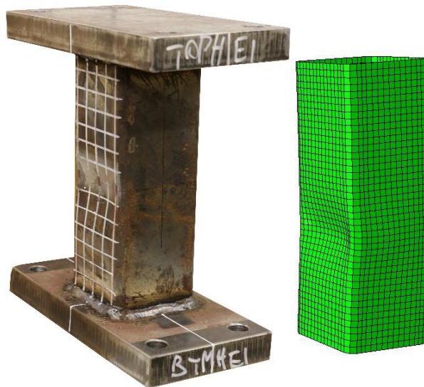
(b) Section yielding failure mode (H80×80×4-BC-e80)
