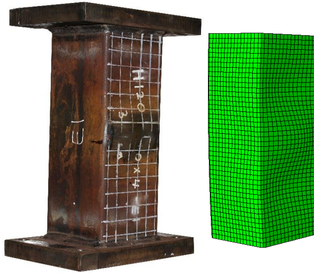
(a) Local buckling failure mode (H120×120×4-BC-e30)
