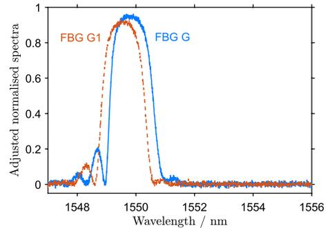
The reference FBG G1 works in reflection mode. The measurement FBG G is subjected to strain (the illustrative environmental factor measured in this paper) and works in transmission mode. This is discussed further in Sects. 3 and 4.
