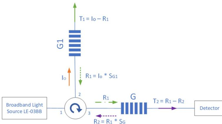
**Fig. 1** Schematic of the measuring system proposed, together with arrows which indicate rays considered in the calculation of the power detected by the detector. G1 is a reference FBG; G is the sensing FBG which in the present implementation is strained
