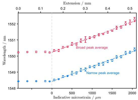
position of a secondary peak, which proved easier to determine as the peak was narrower. Each plot in Fig. 5 shows the average and standard deviation of five measurements. FBG G was not removed from the mechanical system between the measurements presented in Figs. 4 and 5 and those presented for the proposed system when using FBG G in Sects. 4 and 5.
