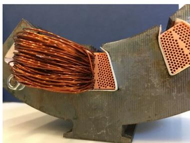
**Figure 4.** One wound coil in the experimental motorette with the slot former inserted.
