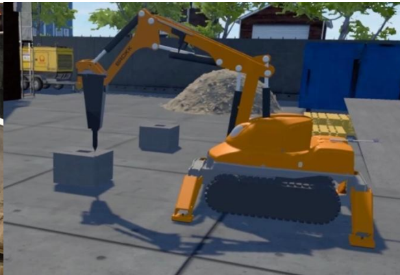
Fig. 1b. Simulated Brokk demolition robot
