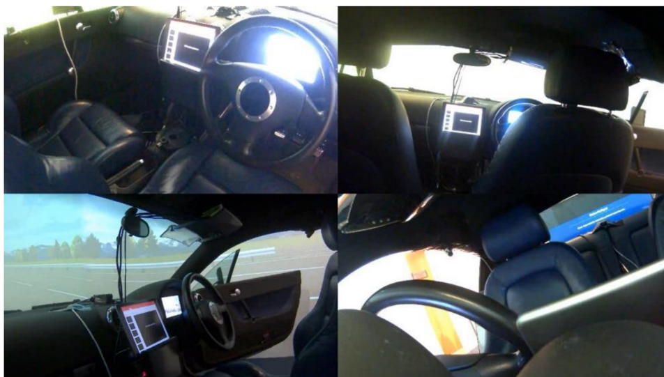
FIGURE 3 Medium-fidelity driving simulator, showing four camera views with iPad (HMI) located in centre console. HMI, human–machine interfaces.
