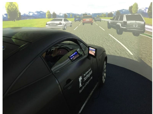
FIGURE 2 Medium-fidelity fixed-base driving simulator.
