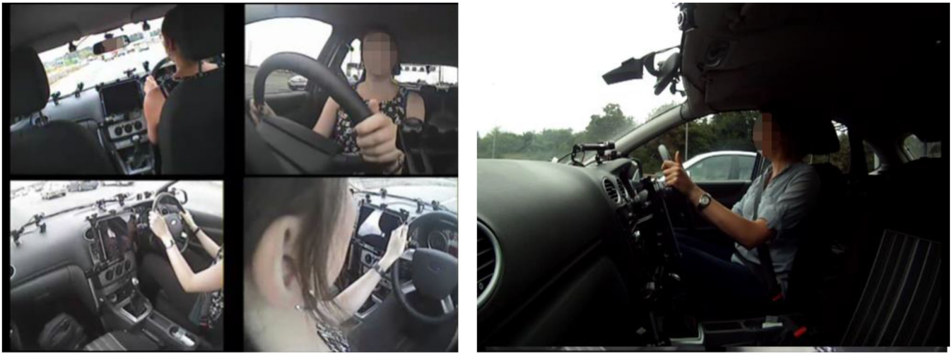
FIGURE 1 Experimental setup in the instrumented car, showing the iPad fixed to the centre console and four bullet camera views (left) and driver seated in vehicle (right).
