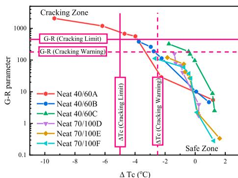
**Figure 6.** Cracking criteria of different methods.
