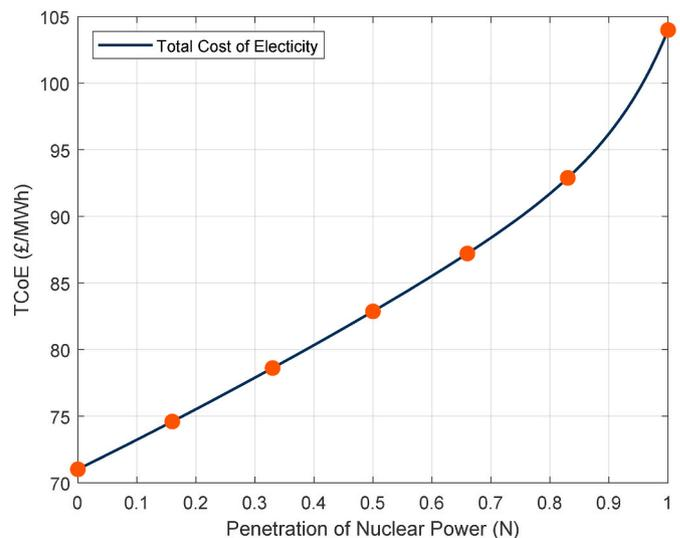
Fig. 15. Relationship between the total cost of electricity and the penetration of baseload nuclear power.
