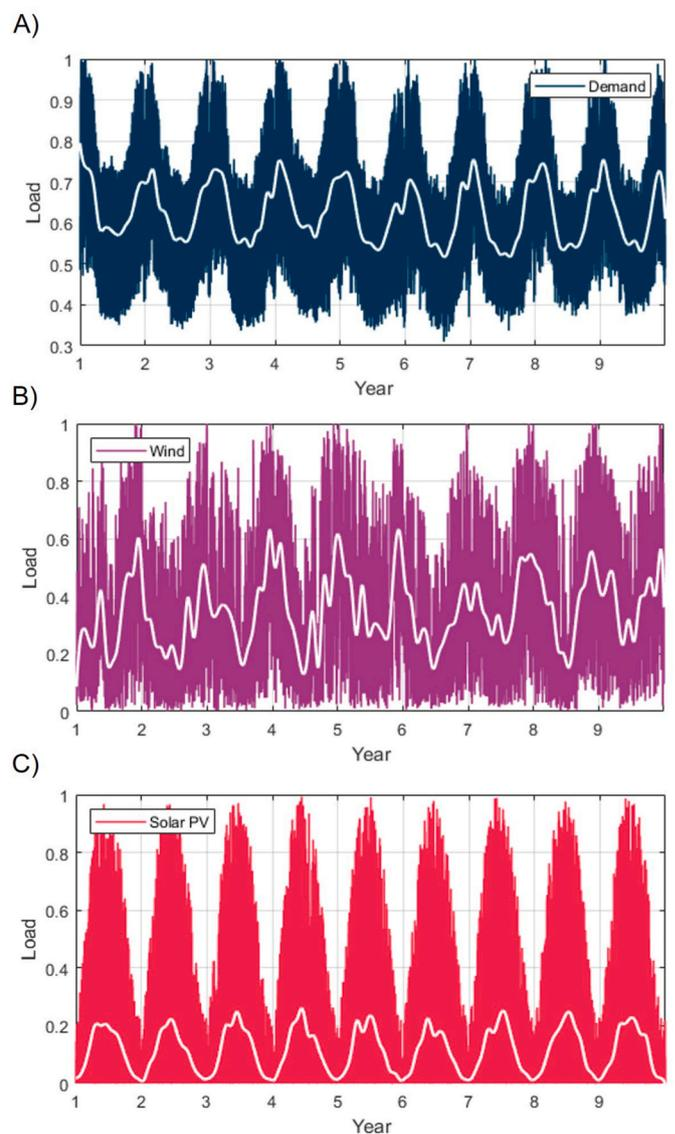
Fig. 1. Normalised profiles containing 9-years of UK data: A) electricity demand [47,48] B) Wind power generation [47,48] C) Solar-PV power generation [49,50].
