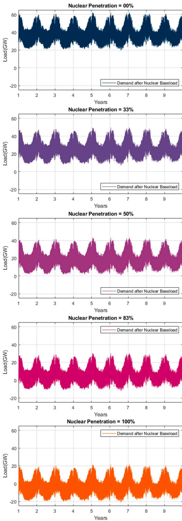
Fig. 9. Profile of demand remaining after nuclear baseload for different levels of nuclear penetration.
