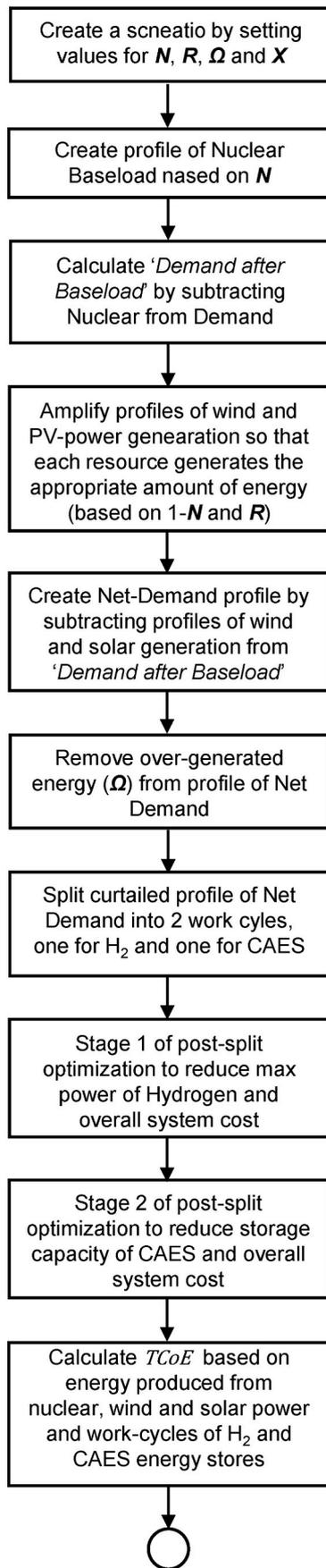
Fig. 2. Algorithm followed to calculate the total cost of electricity achieved by a specific system configuration.
