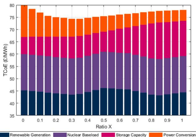
Fig. 8. Breakdown of the total cost of electricity for a system based on  $N = 0.16$  and  $R = 0.9$ .
