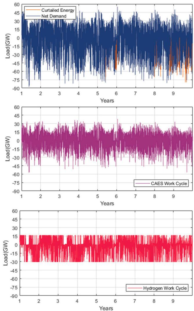
**Fig. 3.** Example of profile of net demand and work cycles for the medium (CAES) and long-duration (H<sub>2</sub>) stores. This scenario considers  $N = 0.16, R = 0.9, X = 0.33$  and  $\Omega = 0.05$ .
