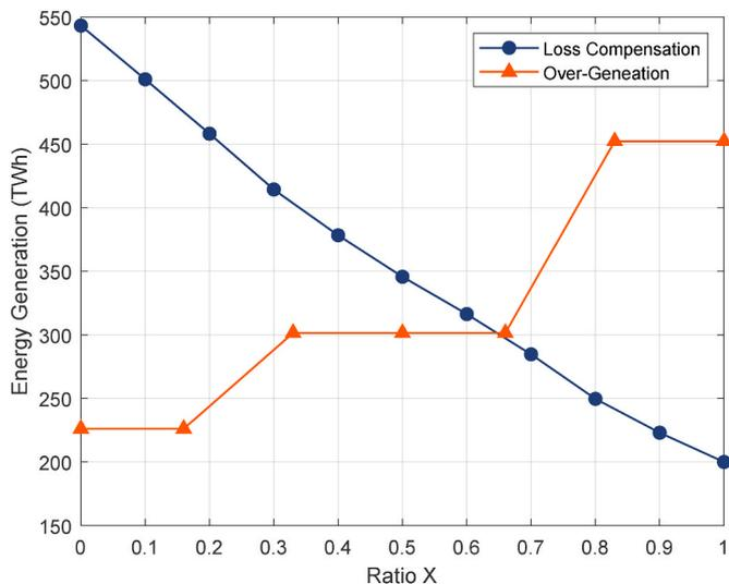
Fig. 5. Behaviour of additional components of renewable generation (loss compensation and over-generation) with respect to  $X$  for  $N = 0.16$  and  $R = 0.9$ .
