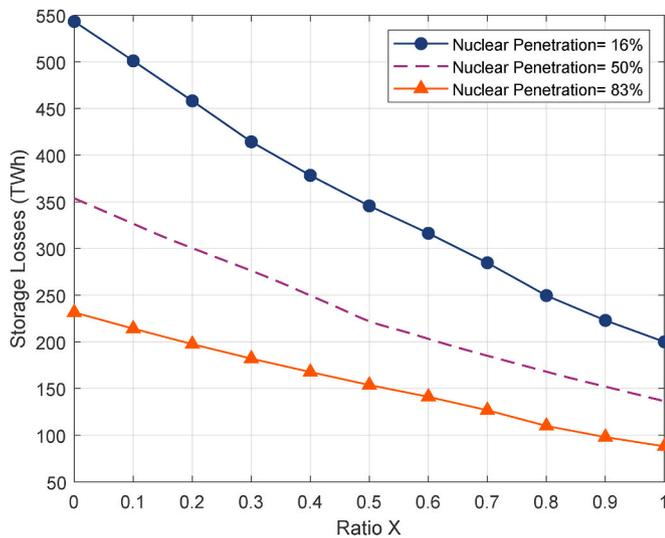
Fig. 13. Effect of nuclear baseload on the overall storage losses (optimum values of  $R$  and  $\Omega$  considered).
