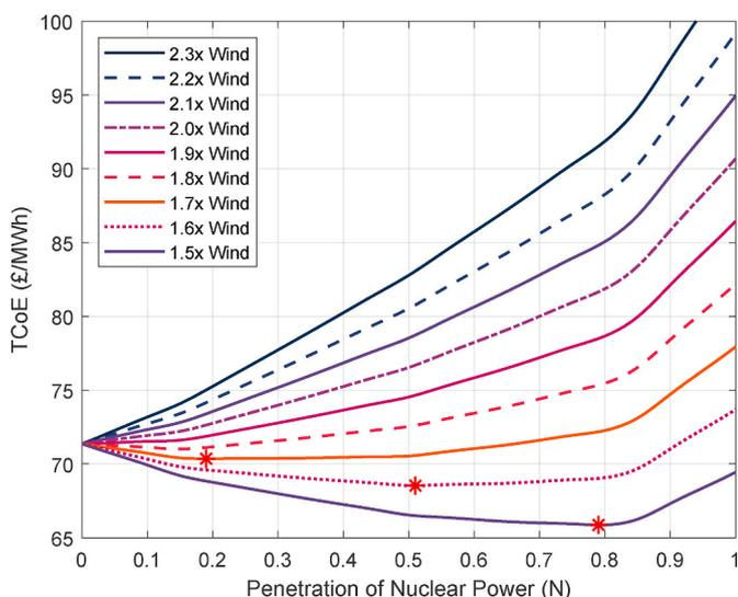
Fig. 16. Effect of a reduction in the cost of nuclear power on the total cost of electricity.
