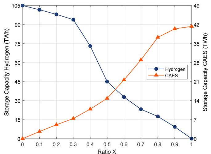
Fig. 6. Energy storage capacities required for different values of  $X$  ( $N = 0.16$  and  $R = 0.9$ ).
