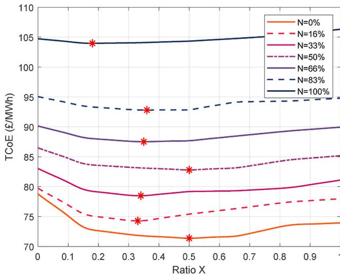
Fig. 14. Variation of the total cost of electricity with respect to penetration of conventional nuclear and storage mix.
