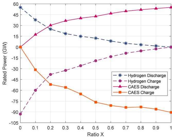
Fig. 7. Behaviour of the charge and discharge powers of both energy stores with respect to  $X$  ( $N = 0.16$  and  $R = 0.9$ ).
