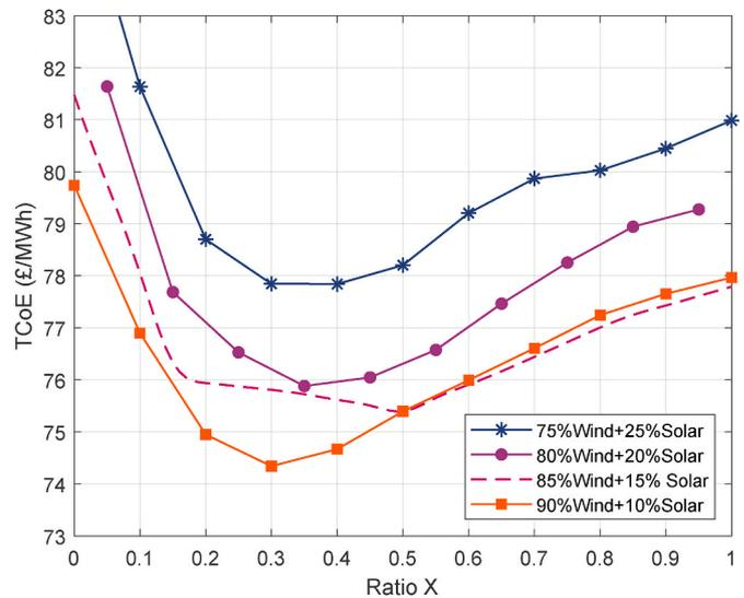
Fig. 4. Effect of different mixes of renewables and energy storage technologies on the total cost of electricity for a system considering a nuclear baseload of 16%.
