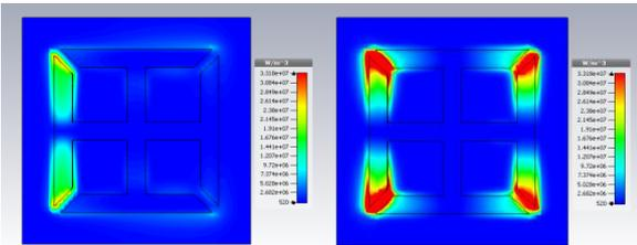
Figure 3. Ohmic loss of single band structure at two different resonance frequencies (left 8.02 GHz), (right 11.31 GHz)
