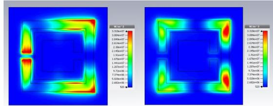
Figure 4. Ohmic loss of single band structure at two different resonance frequency (left 8.02 GHz), (right 11.31 GHz)
