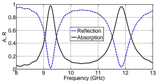
Figure 6. Absorption, reflection and cross wave with Y-polarization
