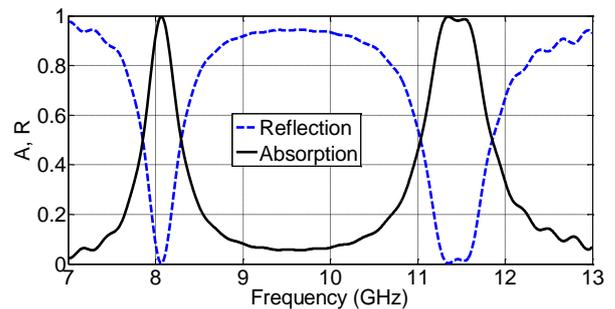
Figure 5. Absorption, reflection and cross wave with X-polarization
