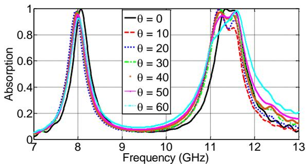
Figure 7. Oblique incidence ( $\theta$ -variation) for variation of E-field at constant Phi ( $\phi = 0$ ) angle
