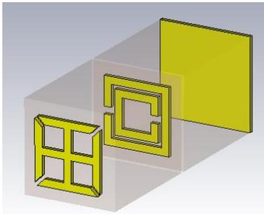
Figure 2. The unit cell composed of two different SRRs
