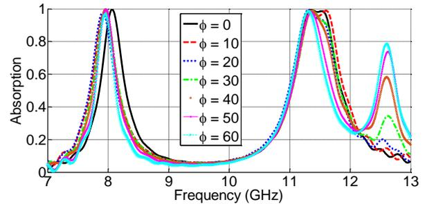
Figure 8. normal incidence for variation of E-field along Phi ( $\phi$ ) for constant Theta ( $\theta = 0$ ) angle
