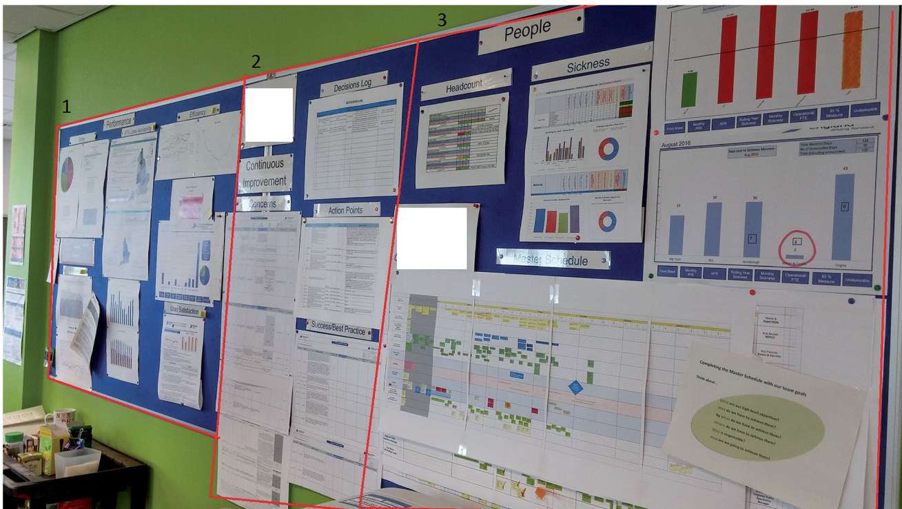
Figure 3. A Type II CI cell board. It has a more systematic focus on work improvement with the 3C process (section 2), alongside work planning and coordination. Team KPIs (section 1) and Human Resources related information (section 3) can also be found on those boards.
