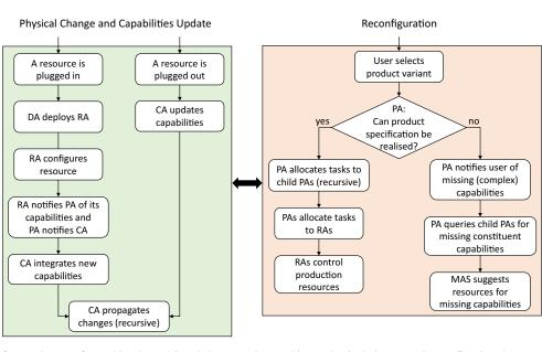
Fig. 3 Sequence of operations performed by the MAS and the user when making a physical change and reconfiguring the system. Capabilities are updated following the bottom-up approach
