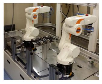
Fig. 6 Reconfigurable production system for assembling detent hinges
