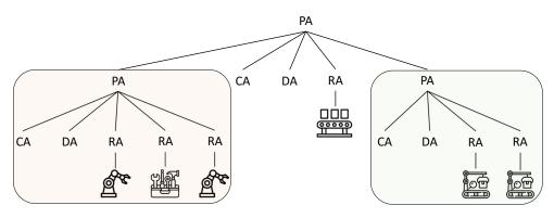
Fig.2 The structure of the MAS used in the experimental evaluation. There are two levels of PAs: the two PAs below the root PA control the two subsystems below them (in coloured boxes). The resources of the subsystem on the left are two robots and a tool changing rack. The resources of the subsystem on the right are two inspection devices. The resource immediately below the root PA is a transport system to move parts between the two subsystems
