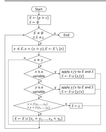
**Fig. 4** Algorithm for matching an operation p in a product specification and a capability c. The output is the most general unifier of p and c if it exists,  $\perp$  otherwise
