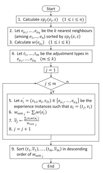
**Fig. 5** Algorithm for the voting scheme for ranking adjustments when k > 1. The input is experience instances  $e_1, \ldots, e_n$  ( $k \le n$ ), a machine state *s*, a performance function *f*. The output is a ranked list of adjustments  $(t_i, v_i)$  ( $i \le m \le k$ )
