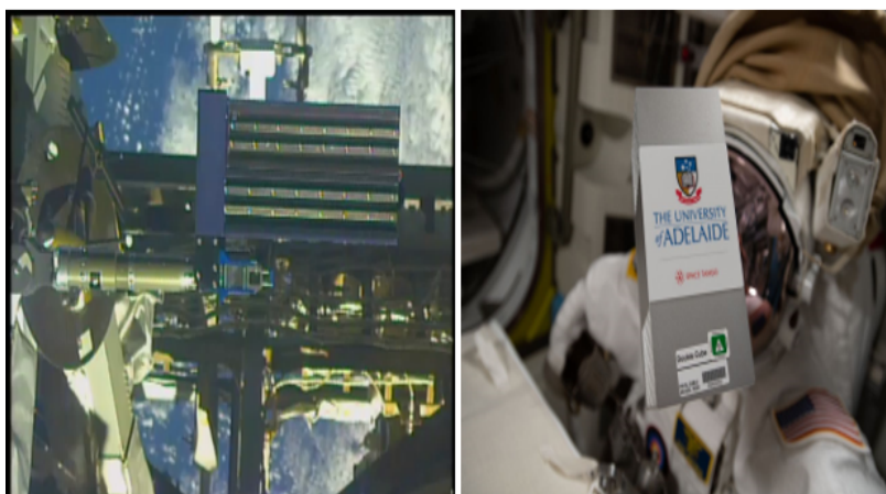
Figure 14 (left) MISSE-14 installation on the MISSE-FF lifting the long-duration cosmic-ray stability experiment of the University of Adelaide towards outer space
