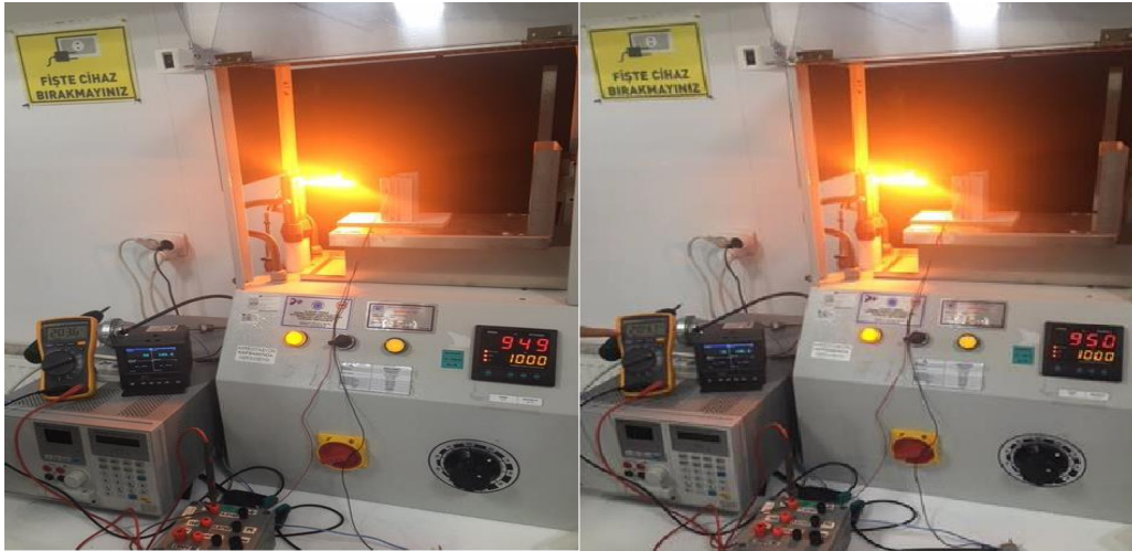
Figure 5: Cell temperature and voltage values at 949 ° C and 950 ° C source temperature
