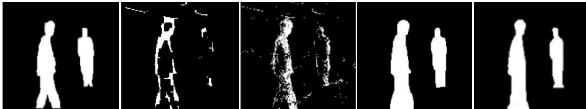
(a)Ground Truth (b) Frame difference method (c) Background subtraction (d)RPCA (e) The algorithm in this paper
