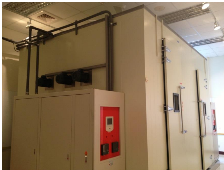
Figure 2: Building insulation performance testing equipment.
