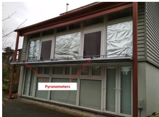
Figure 3: External view of the south façade of the dwelling with the location of the pyranometers. Most glazed areas were covered to minimise the effect of solar radiation
