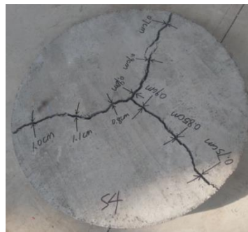
Figure 3: The failure form of hybrid fiber shotcreting panel S4
