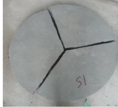
Figure 2: The failure form of plain shotcreting panel S1
