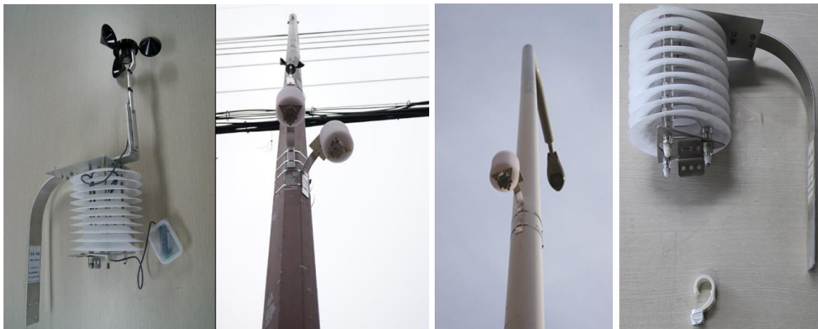
Figure 1: Radiation shield, hook and lamppost for air temperature and wind speed
