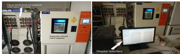
Figure 6: Lithium-ion battery fast charge and discharge test platform
