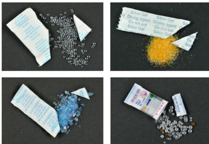
Figure 2: Non-indicating silica gel (upper left), self-indicating silica gel (upper right), partial-indicating (lower left) and non-indicating silica gel with indicator beads (Barbé et al., 2012)
