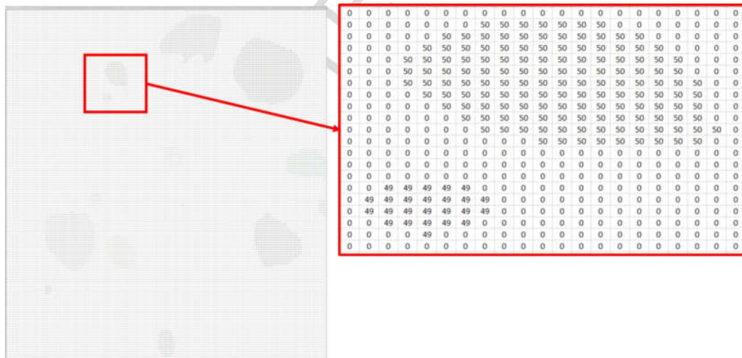
Figure 4. Example of labelled image of bubbles (original image is shown in Figure 3 (a))
