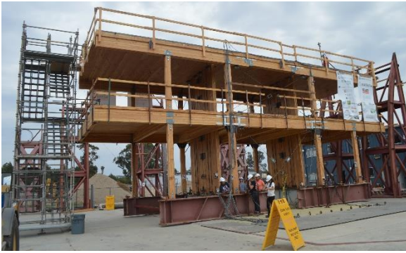
Figure 1: Overview of shake-table specimen tested in 2017. The middle floor level consists of a CLT diaphragm. The roof level consists of a CLT-concrete composite diaphragm.
