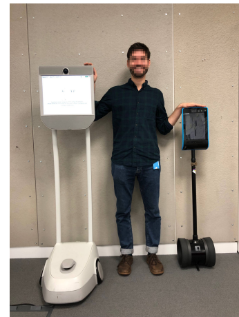
Figure 1: The Beam (left) and Double (right) robots next to a person for size comparison. The Beam has a height of 134.4cm whilst the Double’s height can be adjusted from 119cm up to 150cm.
