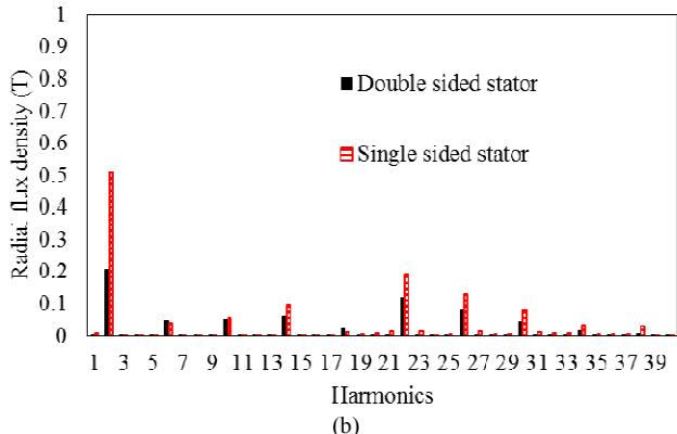
Fig. 4. (a) Inner rotor, and (b) outer rotor radial airgap flux density distribution and harmonics of the single and double-sided stator machines.
