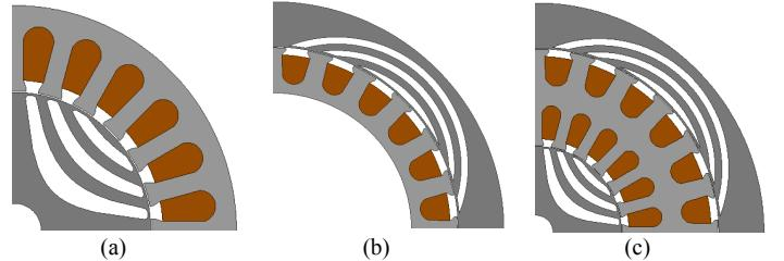
Fig. 1. Cross-sections (a) conventional (b) outer rotor, and (c) double sided stator double rotor synchronous reluctance machines.
