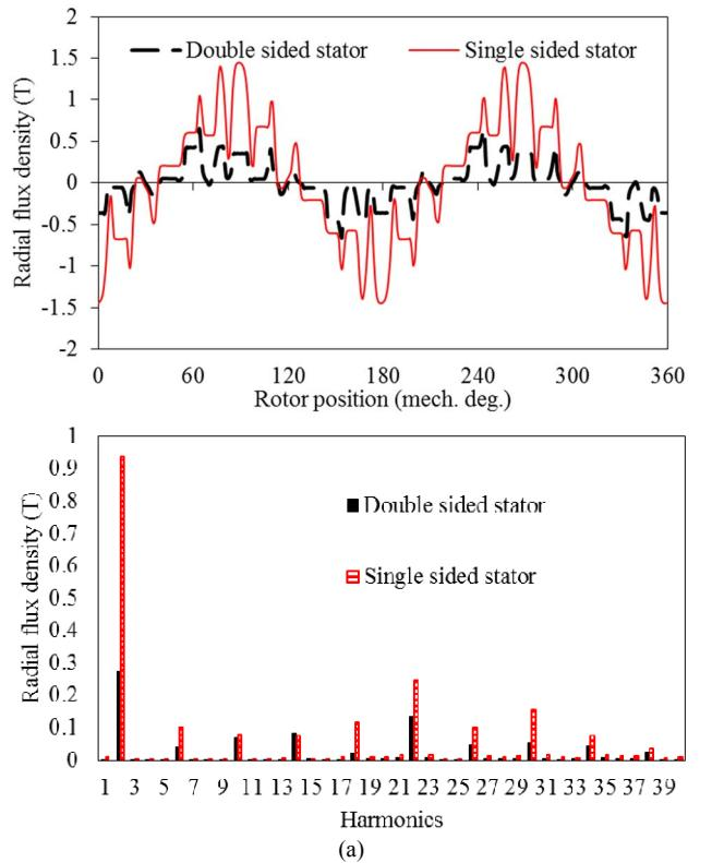
Fig. 4. (a) Line graph of Radial flux density (T) vs Rotor position (mech. deg.) for Double sided stator and Single sided stator. (b) Bar chart of Radial flux density (T) vs Harmonics for Double sided stator and Single sided stator.
