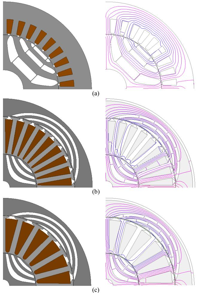
FIG. 5. CROSS-SECTION AND EQUIPOTENTIAL DISTRIBUTION OF (A) CONVENTIONAL SINGLE ROTOR (B) DOUBLE ROTOR WITH 36 SLOTS, AND (C) DOUBLE ROTOR WITH 24 SLOTS.
