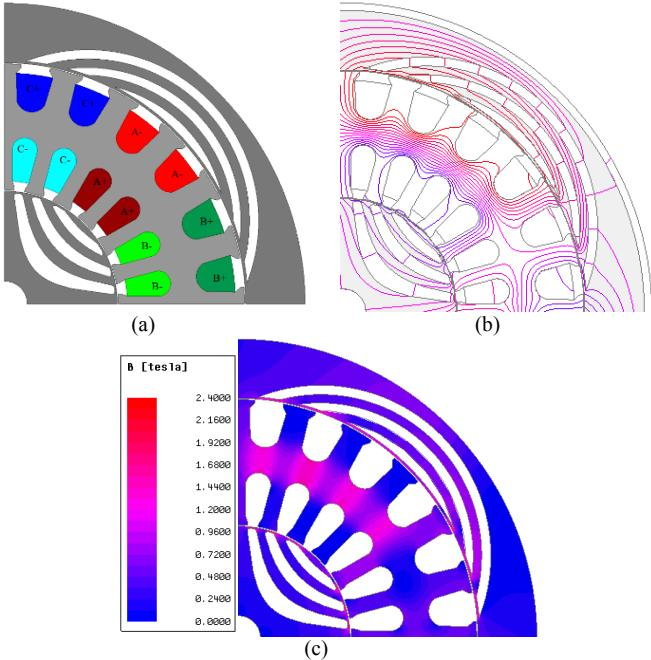
Fig. 2. (a) Cross-section, and (b) equipotential distribution of the radial toroidal concentrated winding configuration of double rotor synchronous reluctance machine with double-sided stator.
