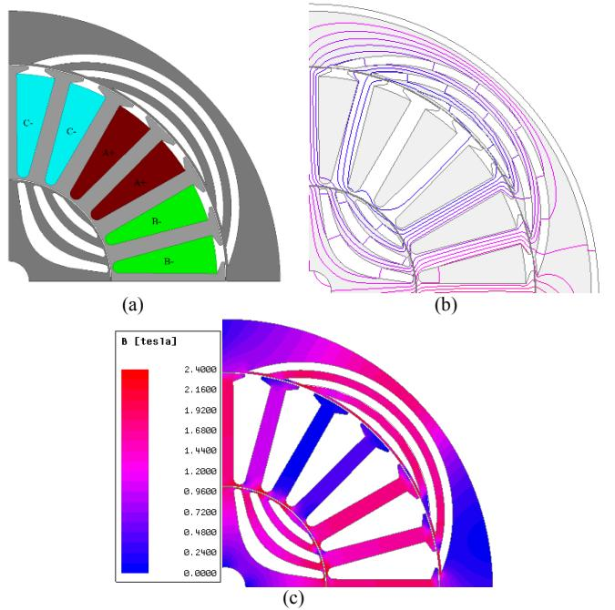
Fig. 3. (a) Cross-section, and (b) equipotential distribution of the distributed winding double rotor synchronous reluctance machine with single-sided stator.
