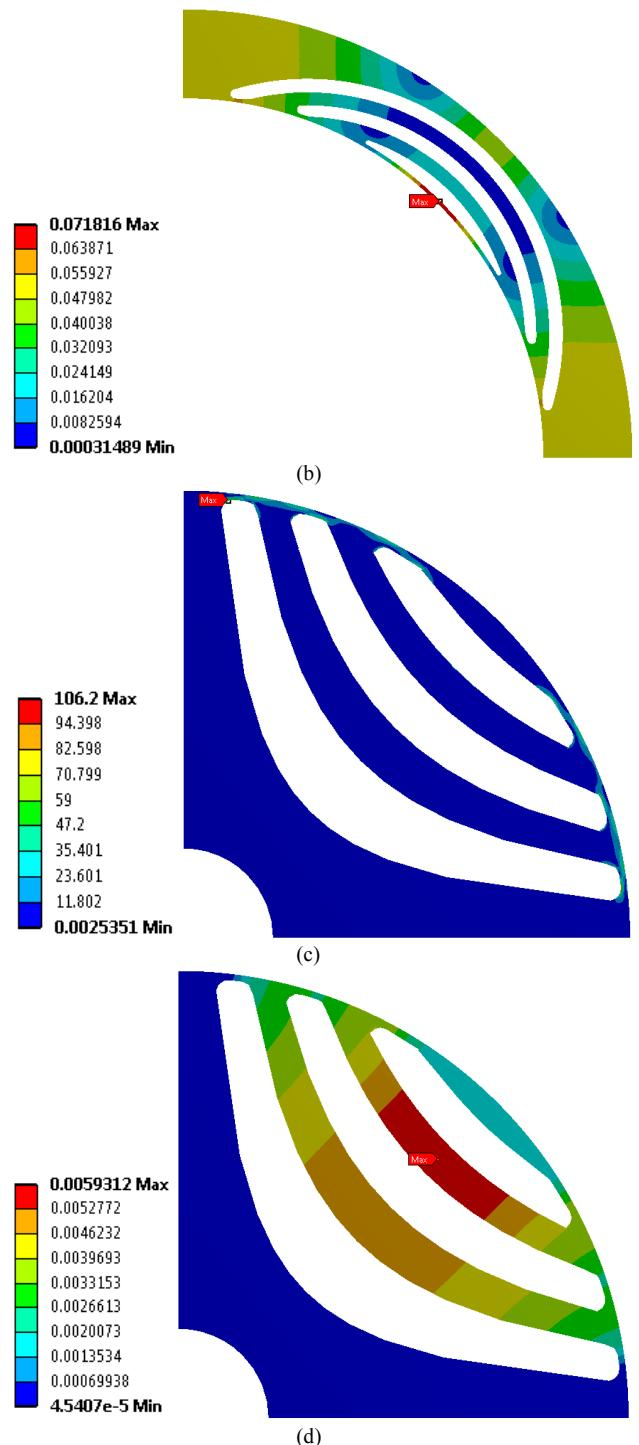
Fig. 8. Mechanical stress and deformation distribution in inner rotor (a) and (b) and outer rotor (c) and (d) of the double rotor machine.
