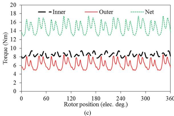
Fig. 7. Torque waveforms of (a) Conventional single rotor (b) Double rotor with 36 slots, and (c) Double rotor with 24 slots.
