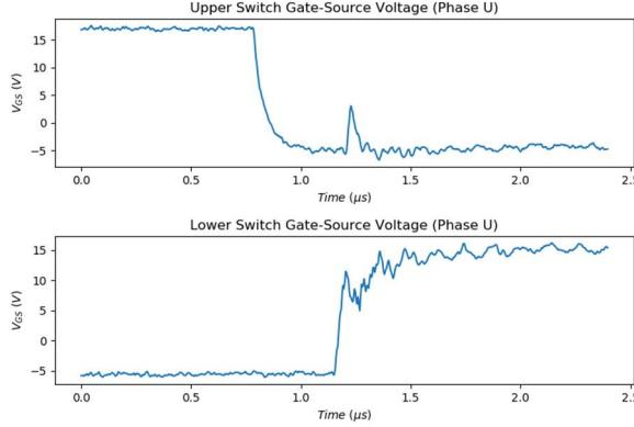
Figure 11a: PCM Phase U MOSFET 10 kHz switching, 375 ns dead-time, negative output current.
