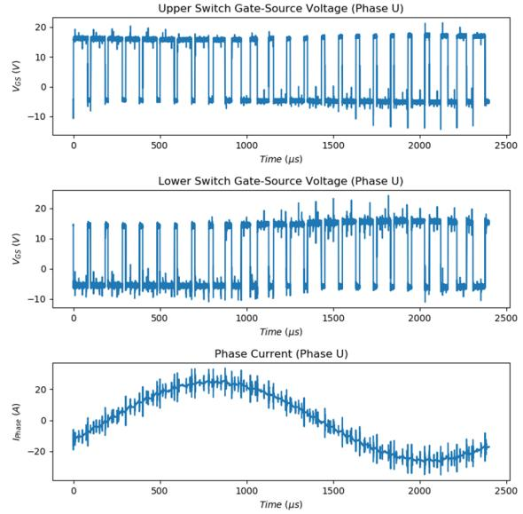
Figure 5b: HPEM Phase U MOSFET switching and output current
