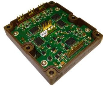
Figure 1b: 5 kVA High Power Electronics Module (HPEM) demonstrator.
