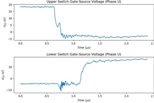
Figure 7a: PCM Phase U MOSFET switching, lower switch turn-on, positive output current
