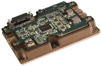
Figure 1a: 5 kVA Power Core Module (PCM) demonstrator.
