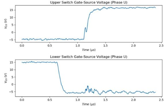
Figure 8b: HPEM Phase U MOSFET, upper switch turn-on, positive output current.
