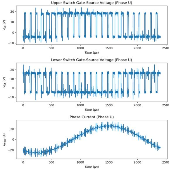
Figure 5a: PCM Phase U MOSFET switching and output current
