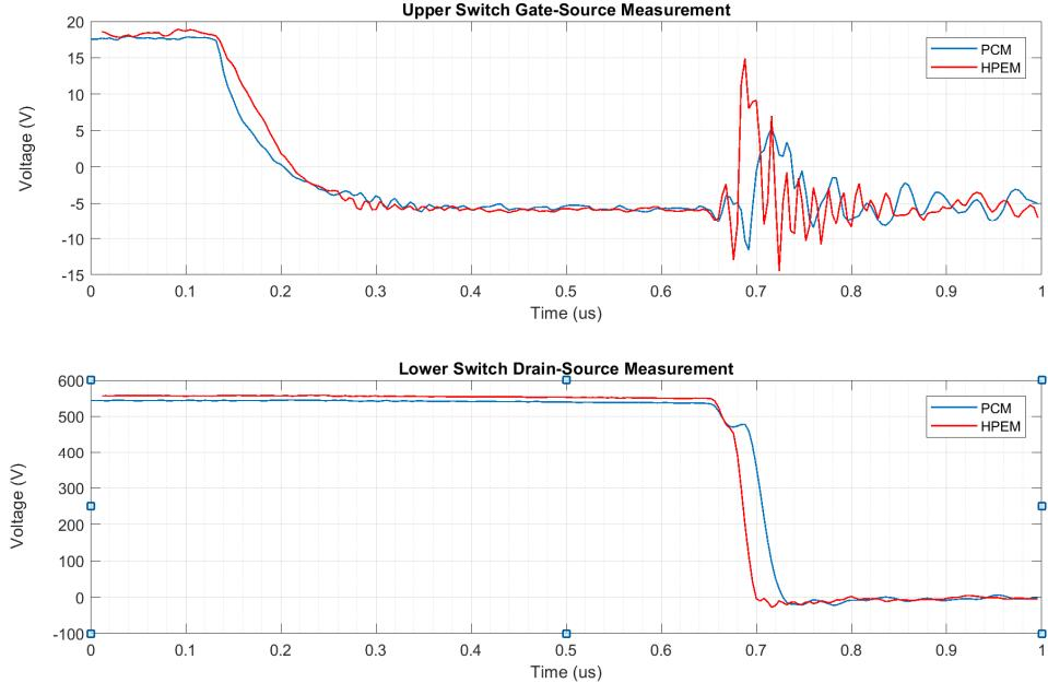
Figure 12: Comparison of PCM and HPEM  $V_{GS}$  and  $V_{DS}$  signals.
