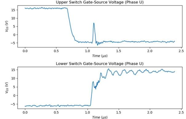
Figure 11b: HPEM Phase U MOSFET 10 kHz switching, 375 ns dead-time, negative output current.
