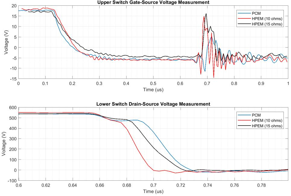
Figure 13: Comparison of PCM and HPEM 10  $\Omega$  and 15  $\Omega$   $V_{GS}$  and  $V_{DS}$  signals.
