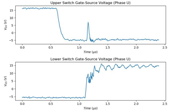
Figure 9b: HPEM Phase U MOSFET 20 kHz switching, lower switch turn-on, negative output current.
