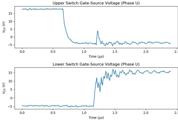
Figure 9a: PCM Phase U MOSFET 20 kHz switching, lower switch turn-on, negative output current.
