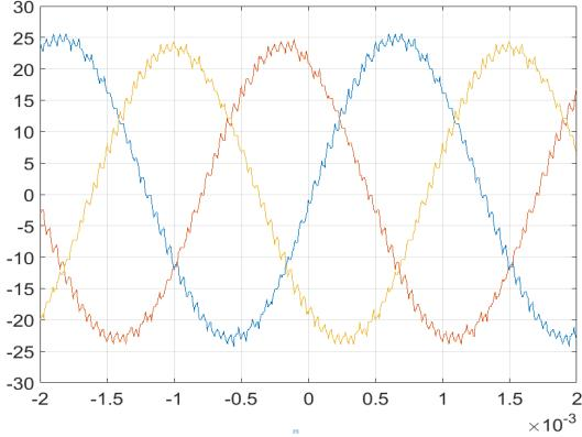
Figure 4a: PCM 3-phase output currents
