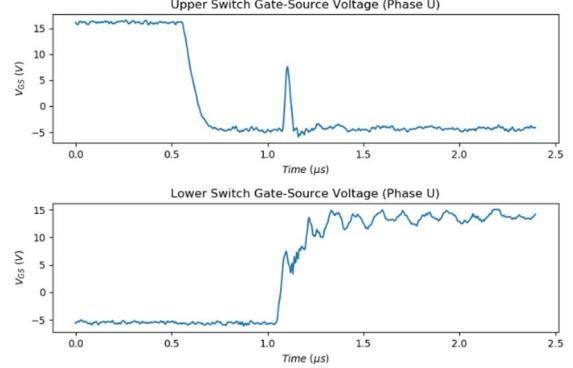
Figure 6b: HPEM Phase U MOSFET switching, lower switch turn-on, negative output current
