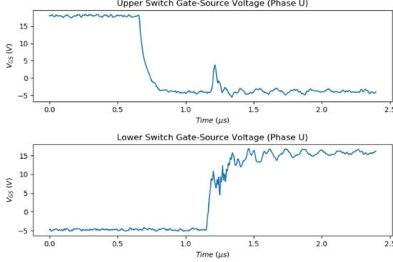
Figure 6a: PCM Phase U MOSFET switching, lower switch turn-on, negative output current
