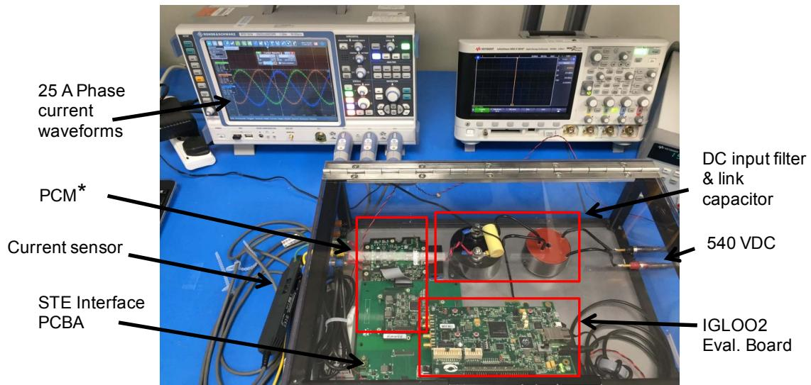
Figure 3: PCM Test Setup
