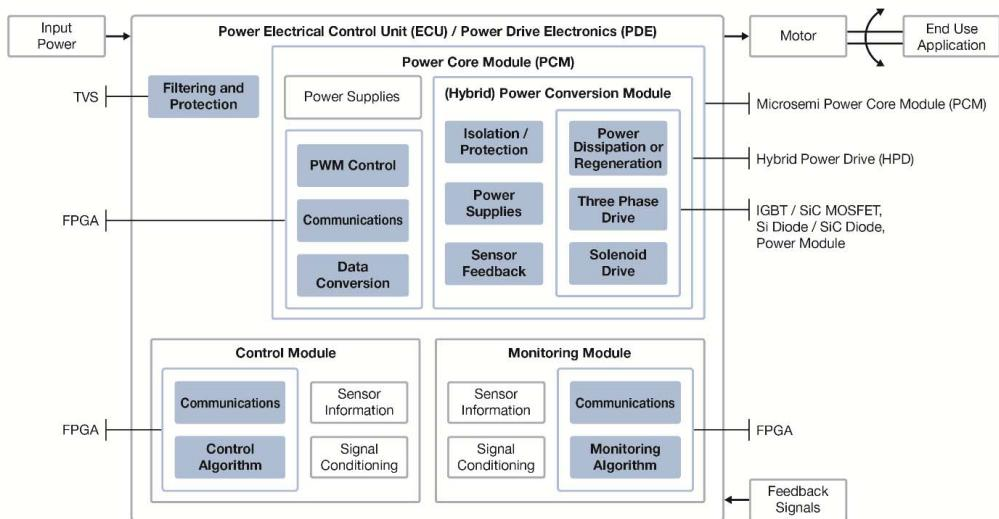
Figure 2: Aviation Intelligent Power Electrical Control System
