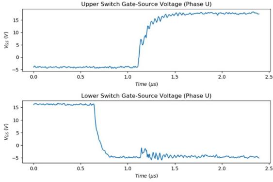
Figure 8a: PCM Phase U MOSFET, upper switch turn-on, positive output current.
