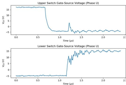
Figure 10a: PCM Phase U MOSFET 50 kHz switching, lower switch turn-on, negative output current.
