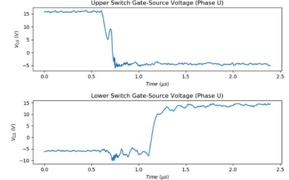
Figure 7b: HPEM Phase U MOSFET switching, lower switch turn-on, positive output current
