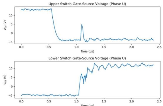
Figure 10b: HPEM Phase U MOSFET 50 kHz switching, lower switch turn-on, negative output current.
