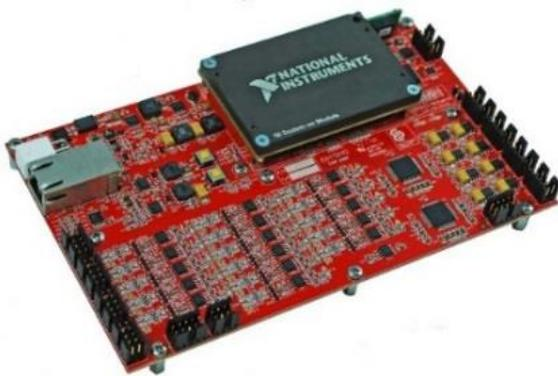
Figure 6. PED-Board control unit.
