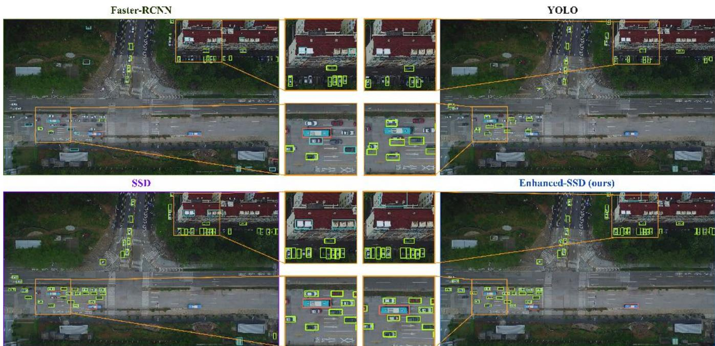
Fig. 10. Counting results on testing image 2 using four deep learning approaches. True positives (correctly detected vehicles) are marked using green boxes with corresponding class types and confidence scores, while false positives (erroneous detections) are denoted using red boxes and false negatives (missed vehicles) are surrounded by orange boxes.
