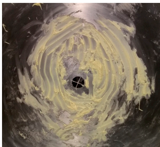
Figure 6. Deposited white chocolate fouling.
