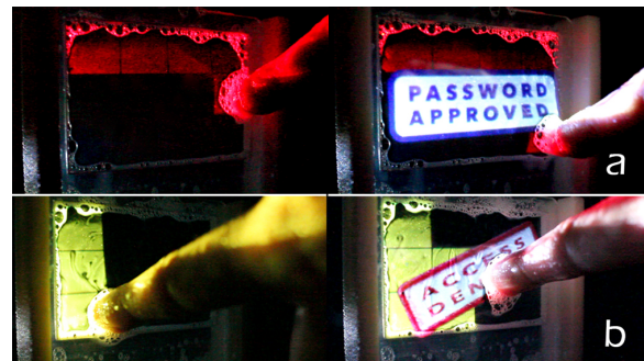
Figure 5. (a) A user unlocks the passcode by drawing a correct pattern on the film with correct depth (indicated by color). (b) Access denied by drawing a wrong pattern.
