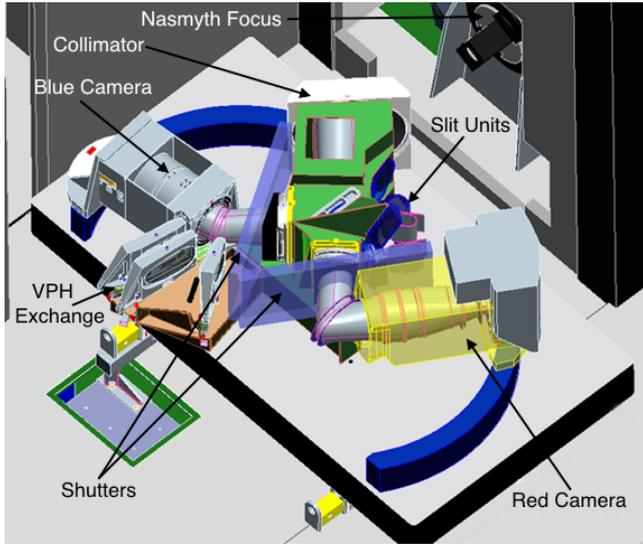
**Figure 3.** A CAD representation of the WEAVE spectrograph installed in the GHRIL instrument room on the WHT Nasmyth platform. The spectrograph cameras are pictured in a configuration unused in practice, with the blue camera at the LR position and the red camera at the HR position. As a scale reference, the optical bench is approximately 3 m long.
