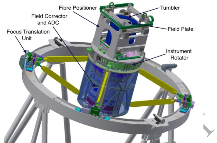
**Figure 1.** A computer-aided diagram (CAD) representation of the WEAVE top-end assembly, incorporating the prime-focus (field) corrector system, instrument rotator and fibre positioner. The four mounting units on the outer ring of the telescope structure provide for focus and tilt correction of the whole system.
