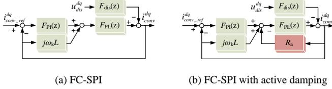
Fig 3. Synchronous reference frame PI controllers
