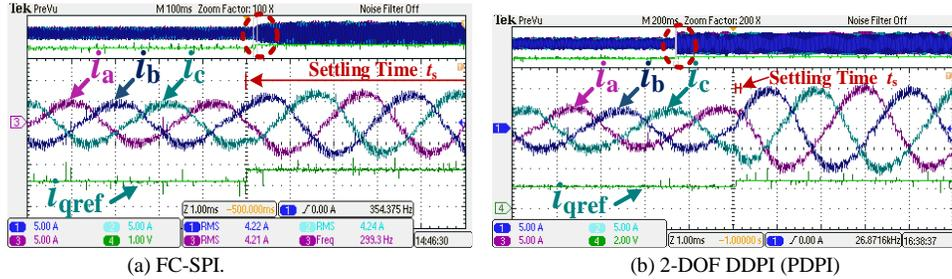
Fig. 13. Dynamic responses comparison at 9krpm, ratio = 33.
