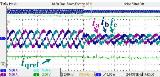
Fig. 17. Transient responses of PDPI at 12krpm, ratio = 25.
