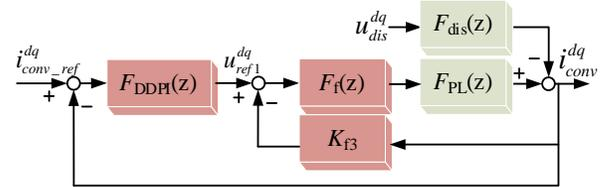
Fig. 5. 2-DOF discrete PI current controller
