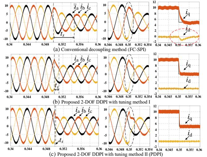
Fig 11. Transient response at 6000rpm, ratio = 50.
