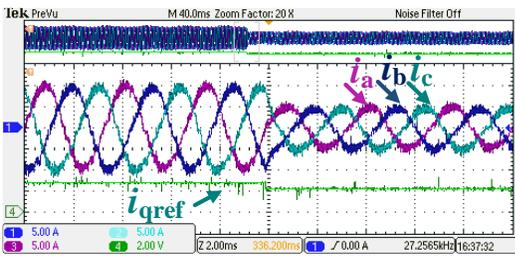
Fig. 16. Transient responses of PDPI at 9krpm, ratio = 33.
