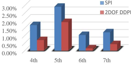
Fig. 20. Low-order harmonics component amplitudes comparison between FC-SPI and 2-DOF DDPI (PDPI).
