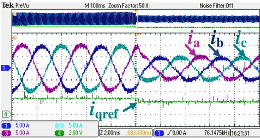
Fig. 15. Transient responses of PDPI at 6krpm, ratio = 50.
