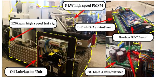
Fig 10. Experimental test platform.
