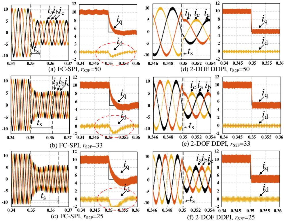
Fig. 12. Transient response comparison between FC-SPI (left) and proposed PDPI (right) with varied S2F ratios.
