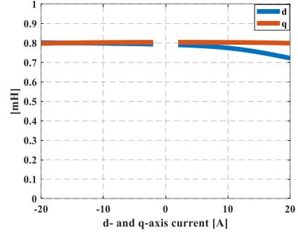
Fig 9. Machine inductance corresponding to different current.
