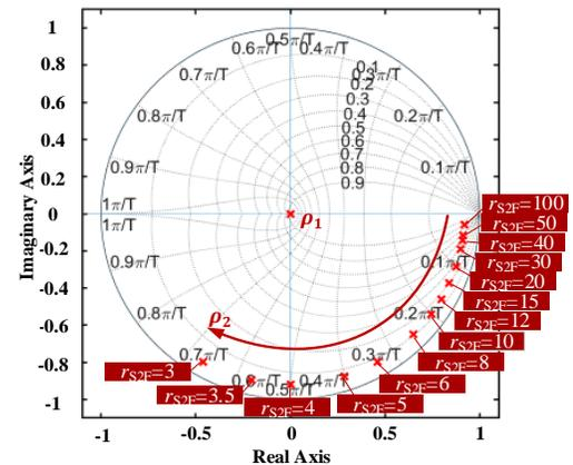
Fig. 2 Pole map of accurate plant model with varied  $r_{S2F}$
