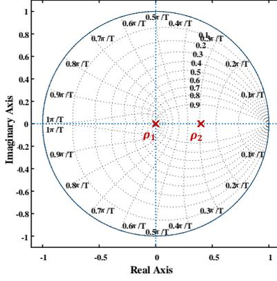
Fig. 6. Pole map of revised inner loop.
