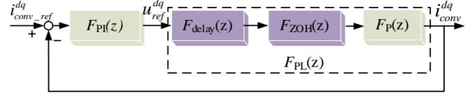
Fig 1. Simplified complex-frame control and plant model
