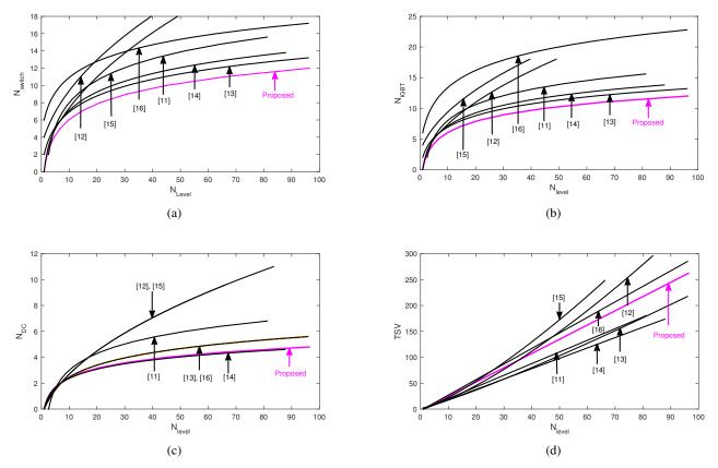
Fig. 3: (a) the variation number of required switches versus  $N_{Level}$ ; (b) the variation number of required IGBTs versus  $N_{Level}$ ; (c) the variation number of required DC power sources versus  $N_{Level}$ ; (d) the variation magnitude of TSV versus  $N_{Level}$ .
