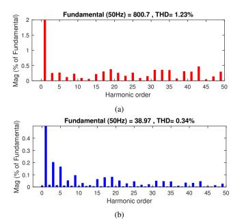
Fig. 6: (a) FFT of the voltage (THDv = 1.23%); (b) FFT of the current (THDi = 0.34%).
