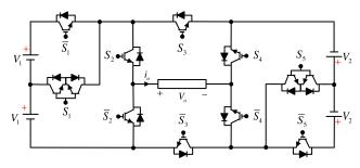
Fig. 1: The proposed 17-level basic inveretr.
