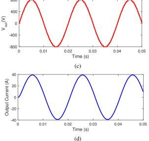
Fig. 5: Simulation studies; (a) 17-level output voltage curve of first unit; (b) 17-level output voltage curve of second unit; (c); 33-level total output voltage curve of the proposed cascaded multilevel inverter; (d) output current curve.
