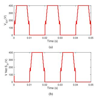
Fig. 7: (a) the maximum blocked voltage by switch  $S_{31}$ ; (b) the maximum blocked voltage by switch  $\bar{S}_{31}$ .
