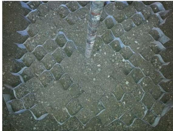
*Fig. 2. A view of geocell spread over the anchor plate in the test pit*
