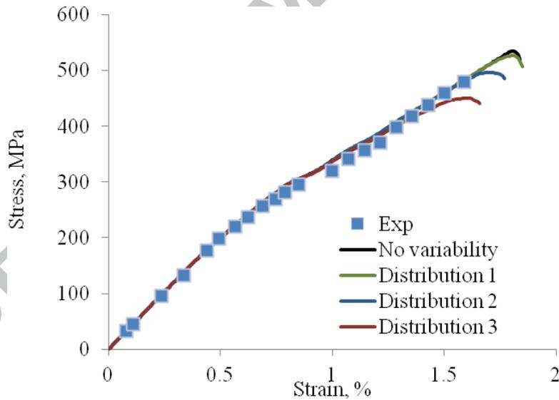
**Figure 4.** Experimental and predicted stress-strain curves (ELS model) for plain weave composite with and without variability; Distributions 1, 2 and 3 are original and widened ( $\times 2$ ,  $\times 3$ ) distributions of fibre strength
