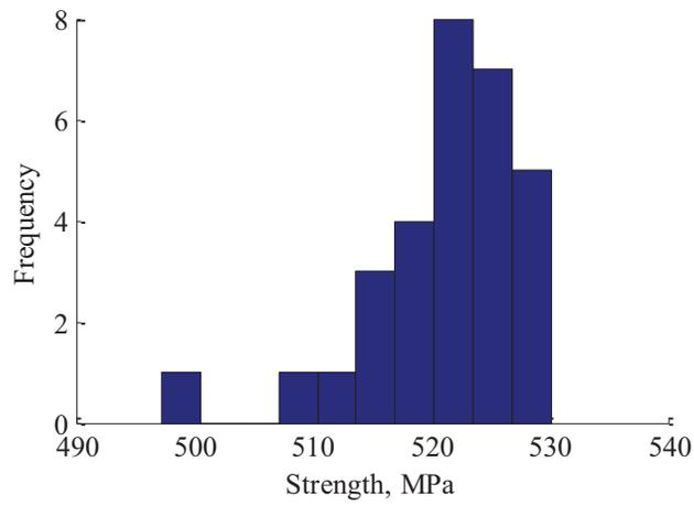
Figure 5. Final strength distribution (30 simulations, ELS fibre bundle model)
