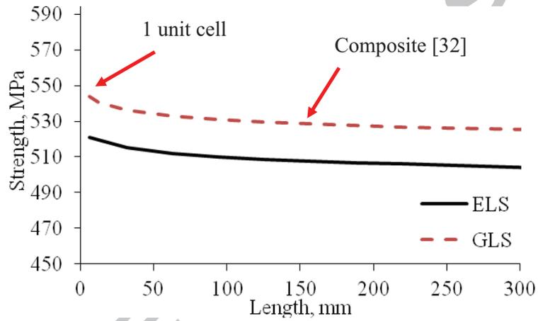
Figure 6. Average strength of the chain of unit cells
