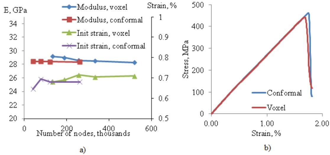
**Figure 3.** a) Convergence of voxel and tetrahedral meshes; b) Comparison of stress-strain curves for voxel and conformal mesh solutions
