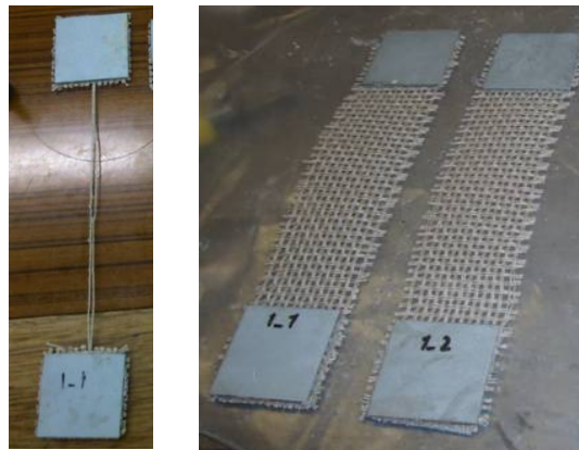
Fig.2 Specimen details for tensile tests: (a) single yarn; (b) fabric test.
