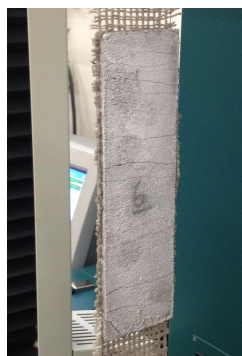
Fig.9 Typical failure mode of the specimens.
