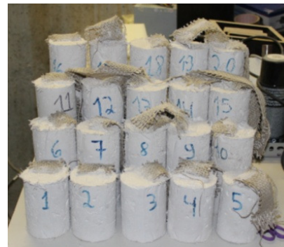
Fig.4 Pull-out test specimens: (a) geometrical details; (b) specimens.
