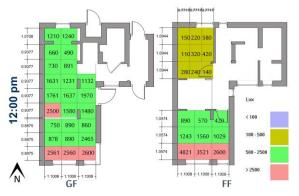
Figure 5: Onsite daylight illumination spotr measurements of all the zones on a clear sky day (10th April 2018 12:00pm)
