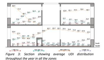
An in-depth climate-based daylight illumination renders were analysed to identify the UDI distribution
