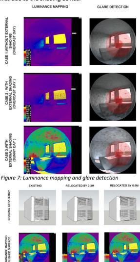
Figure 8: Shading device and Luminance mapping
