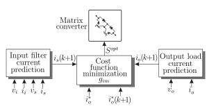
Figure 7. Predictive current control with imposed input current block diagram.
