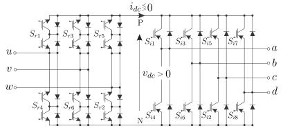
Figure 22. Four-Leg indirect matrix converter.
