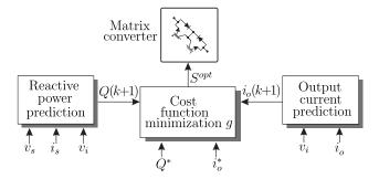
Figure 6. Predictive current control with reactive power minimization block diagram.
