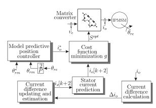
Figure 14. Predictive position and speed control block diagram.
