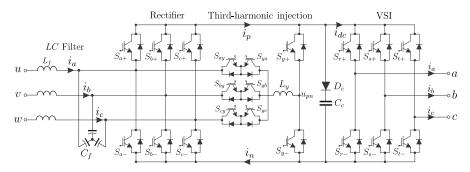
Figure 24. Two-stage matrix converter with third-harmonic injection.
