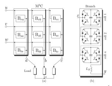
**Figure 20.** Modular multilevel matrix converter. (a) Generic  $M^{3}C$ , (b) Branch composed by one inductor  $L_{B}$  and *n* full-bridges.
