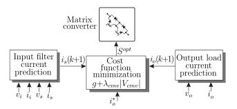
Figure 10. Predictive current control with common-mode voltage block diagram.
