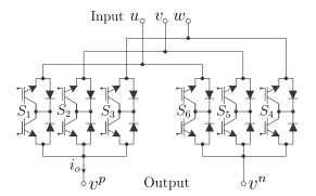
Figure 16. A single-phase matrix converter.
