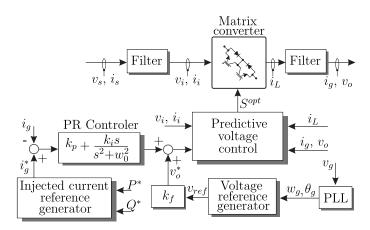
Figure 12. Predictive voltage control block diagram.
