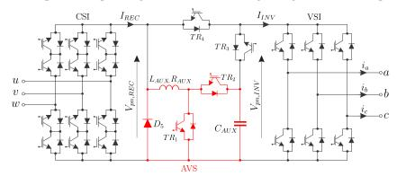
Figure 27. Hybrid indirect matrix converter.
