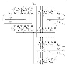
Figure 29. Multi-drive indirect matrix converter.
