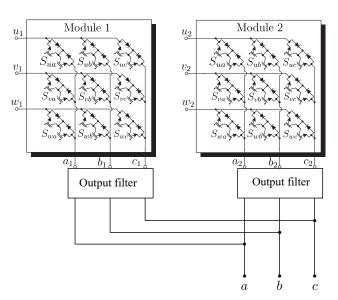
Figure 19. Multi-modular matrix converter.
