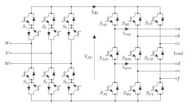
Figure 28. Indirect matrix converter with dual output.
