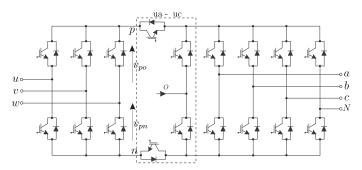
Figure 23. Three-level indirect matrix converter.
