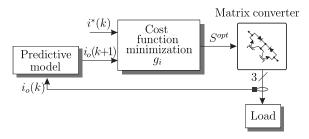
Figure 4. Predictive current control block diagram.
