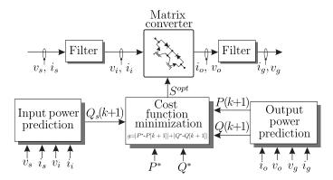
Figure 13. Predictive power control block diagram.
