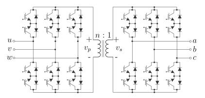
Figure 26. Solid-state-transformer-based matrix converter.
