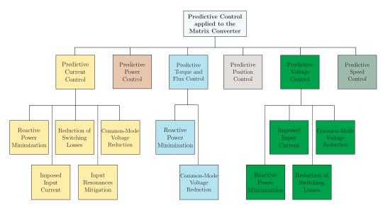
Figure 3. Predictive control techniques applied to matrix converters.
