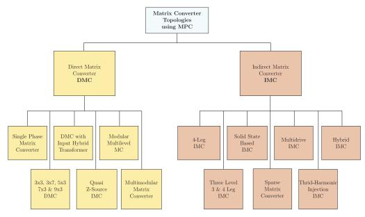
Figure 15. Classification of matrix converters.
