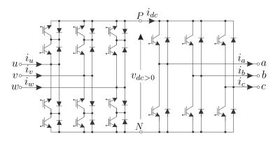
Figure 21. Power stage of an indirect matrix converter.
