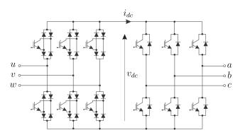
Figure 25. Sparse matrix converter.
