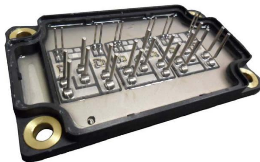
Fig. 1. Multi-chip layout of SiC MOSFET power module [3]
