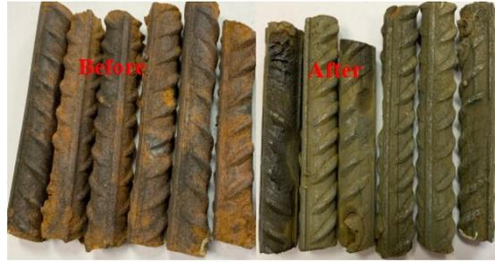
(b) Comparison before and after rust removal
