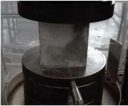
(a) Compressive test of concrete cube
