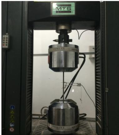
(c) Tensile test of steel bar
