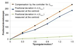
FIGURE 4. Comparison between the actual positional deviations at the centroid of the platform and the compensated values by the controller.
