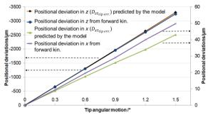
FIGURE 5. Comparison between the target positional deviations predicted by the model and the measured values.
