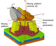
FIGURE 2. Kinematic model of HAMS.
