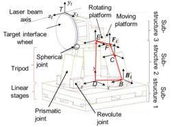
FIGURE 1. Kinematic structure of HAMS.
