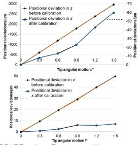
FIGURE 6. Target position accuracy improvement through the calibration process.
