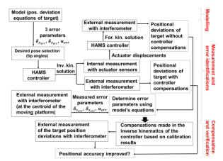
FIGURE 3. The calibration process flow diagram of HAMS.
