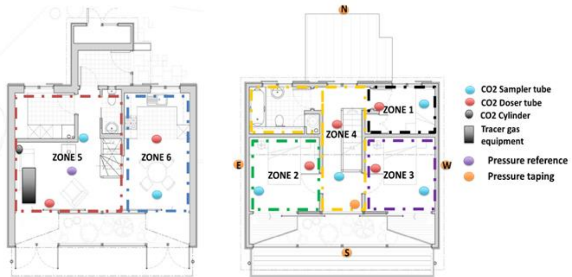
Figure 2. Floor plans of the test house and location of testing devices, left: ground floor; right: first floor.
