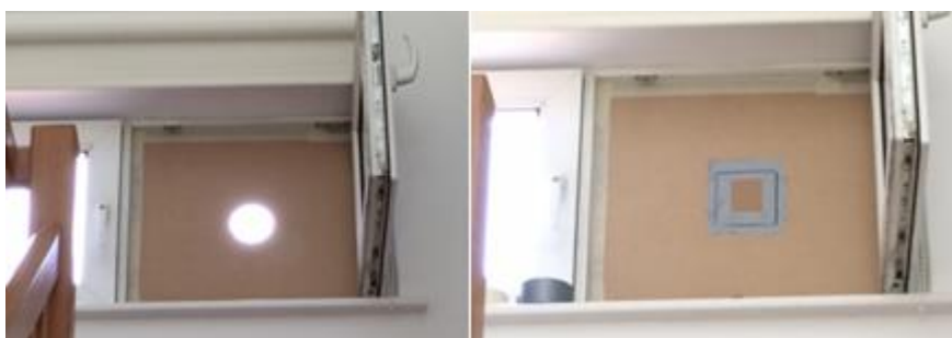
Figure 7: Setup of the known opening in house No. 8
